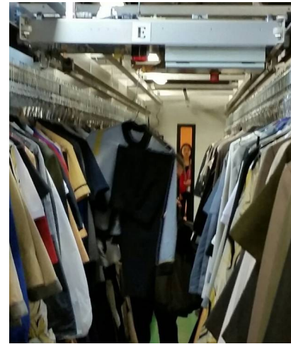
Stored uniforms remain static while an overhead pick-off arm retrieves the requested set
