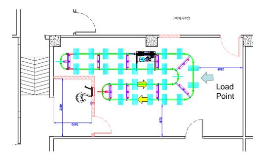
Switch-operated load point for clean uniforms is located at the rear of the conveyor
